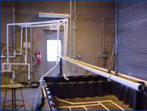
Early Brine Making shop made using PVC piping
