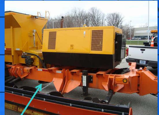
Self-Contained Power Unit For Hydraulics
