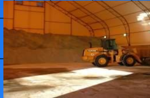
All brine making, storage of both solids and liquids...plus loading...all isolated inside covered building
